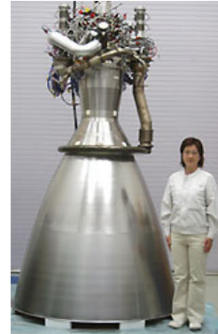
Fig. 11 LE-8 engine (IHI, Japan)[29].
