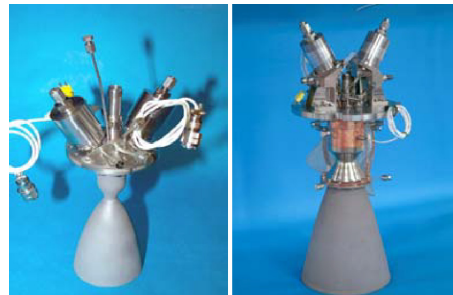
Fig. 7 450 N-class LCH_4/LOx RCS engine developed by Aerojet (left) and Northrop Grumman (right)[19].
