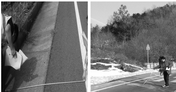
Fig. 2. Measurement of road alignment.
