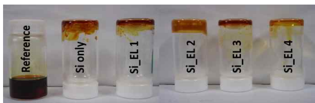
Figure 2. Liquid electrolyte and silica-added gel type electrolytes.
