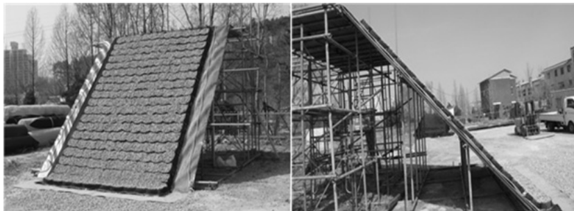
Fig. 8. The test bed for the drainage test of GMC in field
