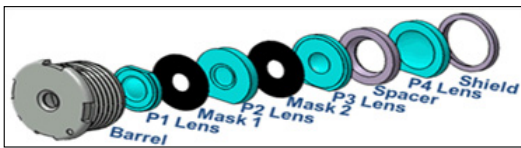
Fig. 2. Structure of lens module
