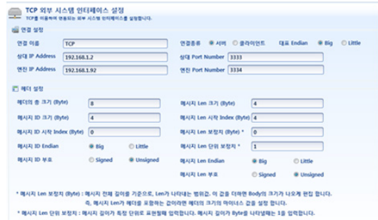
Fig. 9. Configuring GUI for TCP interface block
