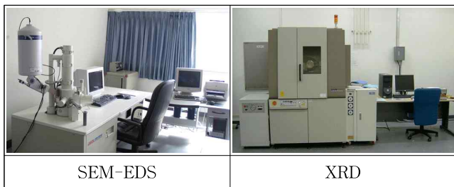
Fig.1 Compositional analysis instruments for efflorescence of traditional bricks
