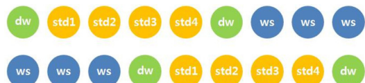
Fig. 4. Sample positions in the autosampler tray for a four-standard arrangement. dw, std and ws stand for dummy water samples (usually, deionized water), standards and water samples to be measured, respectively.
