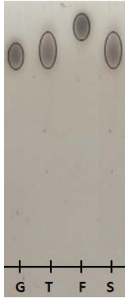
Fig. 8. Comparison of TLC separation of the sample and control monomeric sugars. (G: glucose, T: tetrasaccharide, F: fructose, S: sucrose)
