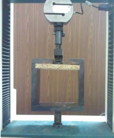
Fig. 3. View of testing arrangement used on screw test.
