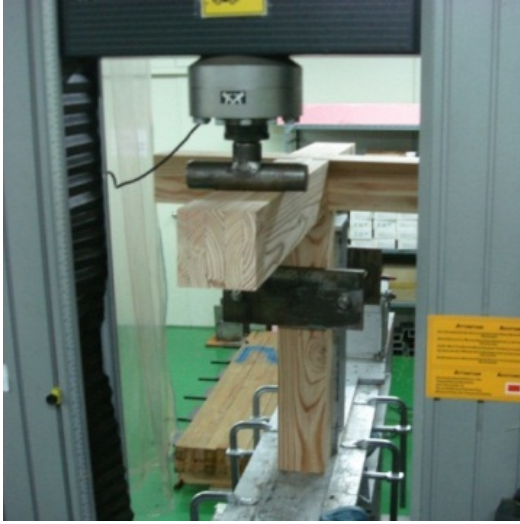
Fig. 1. Experimental test set up for moment carrying capacity of the sagae connection.
