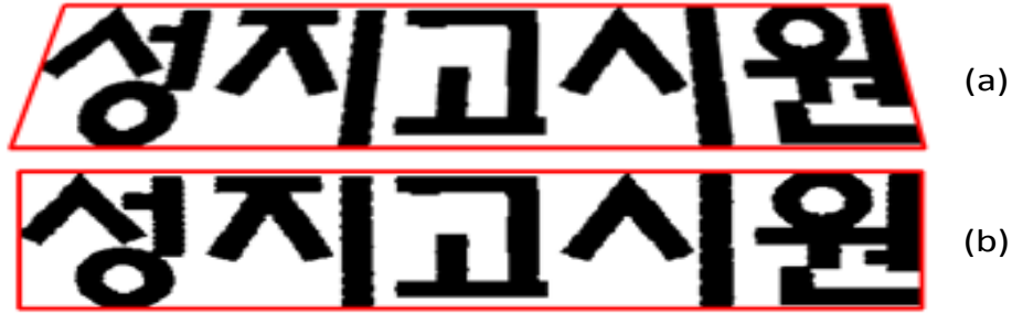
Fig. 8. (a) The trapezoid outline estimated by the proposed method, (b) The results without distortion
