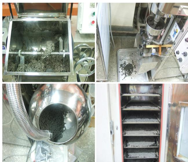
**Fig. 1** Fertilizer manufacturing process using fly ash, bentonite and calcium hydroxide
