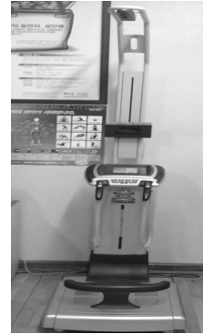
Fig 2. Electrical resistance analyzer (X-SCAN PLUS II)
