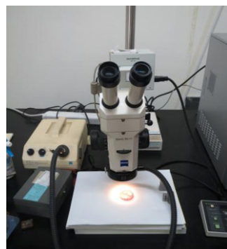
Fig. 5. Stereomicroscope (Carl Zeiss, DE/Stemi SV11, Thornwood, NY, USA) equipped with a digital Olympus DP 10 camera (Olympus, JP/DP 10- PRN, Japan).
