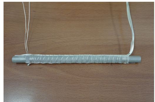
Fig. 2 Cathode current collecting of tubular SOFCs
