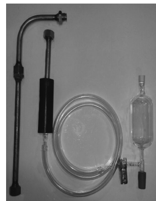
Fig. 2. Image of a Giggenbach bottle connected with a Ti sampling tube.
