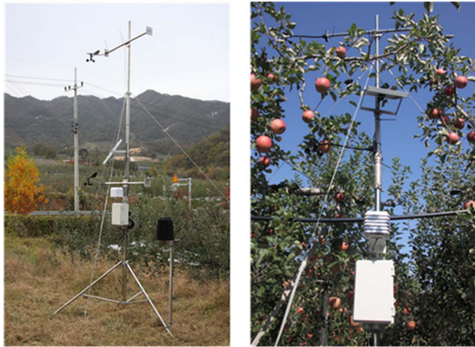
Fig. 3. View of automated weather station installed at the outside (left fig., A station) and inside (right fig., D station) of windbreak net.
