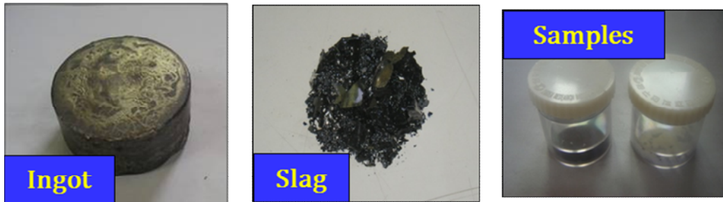
Fig. 4. Representative sample of the radioactive metal waste using melting method.
