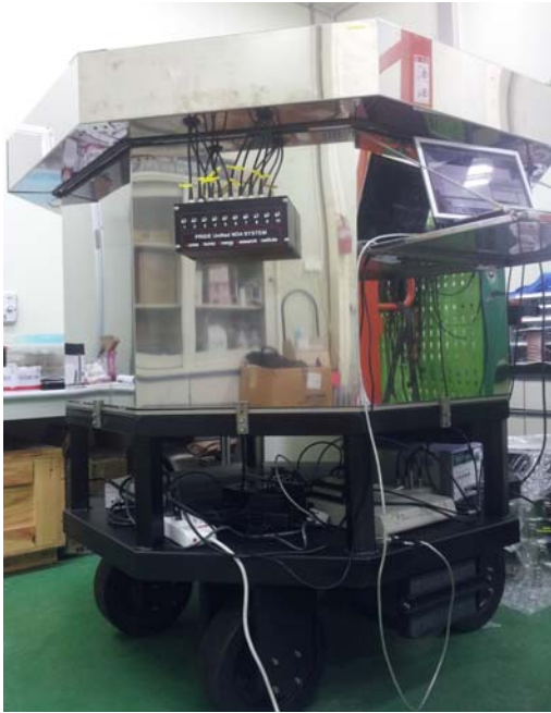
Fig. 1. Unified non-destructive assay system with ^3\text{He} neutron detectors and mass balance.
