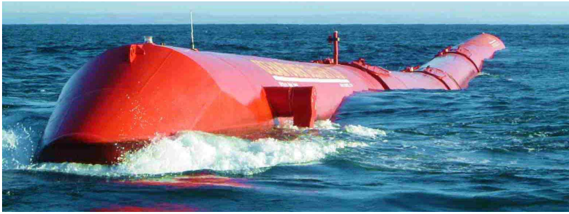
FIGURE 4. View of the Pelamis wave energy converter(image source: www.greenlivinganswers.com)
