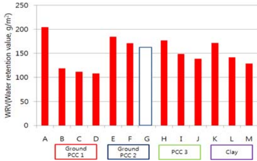
Fig. 3. Effect of pigment blending on the water retention of coating color(WRV of Formula G could not be measured because of color shocking).
