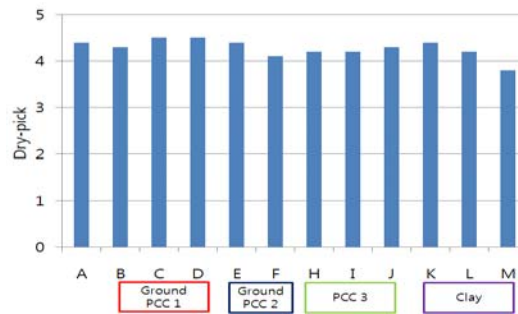
Fig. 9. Effect of pigment blending on the dry-pick strength of coated paper.
