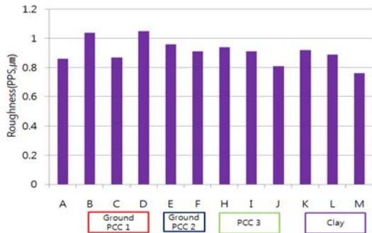
Fig. 4. Effect of pigment blending on the roughness of coated paper.
