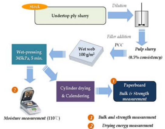
Fig. 2. Flow diagram of the measurements of physical properties and drying energy reduction of duplex-board.
