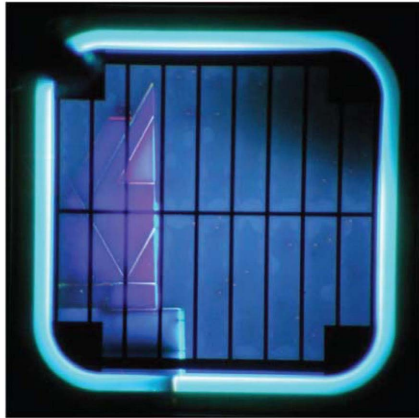
Fig. 4. Real-color electroluminescence image depicting recombination induced SFs (purple triangular features), basal plane dislocations (red linear features), and in-grown stacking fault (blue feature at bottom) within a grid-structured pin diode at 15 mA injection 17)
