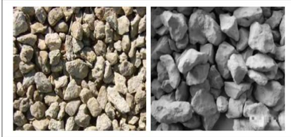
Fig. 7 The feature of recycled aggregate and pre-coated recycled aggregate
