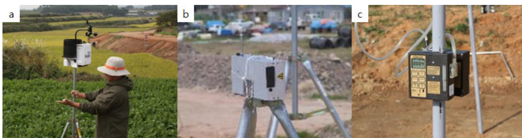
Figure 3 The instruments for measuring of the dispersed aerosols from the road from the livestock transport vehicles; a) portable weather station, b) aerosol spectrometer, and c) air sampler with filter.
