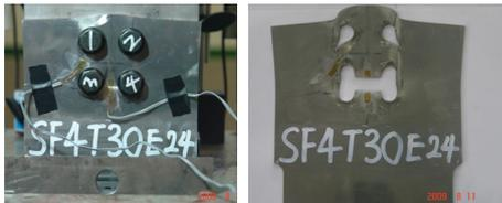
(a) at ultimate strength point / at test finishing point (SF4T30E24)
