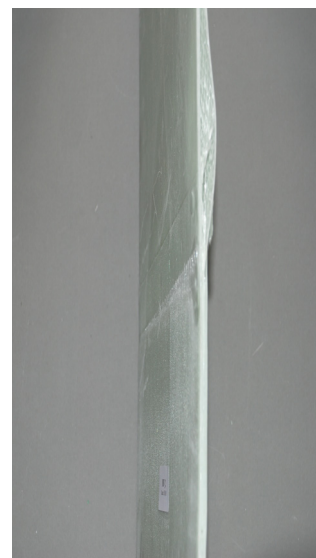
<Fig. 15> Failure mode of connection(MBV_01)
