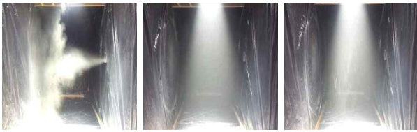
Figure 5. Testing procedure (left to right: spraying demolition dust, waiting for 30 seconds, water spraying)
