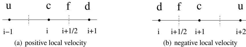
FIGURE 1. Description of face flux nodes according to stream direction: the main purpose of an HRS is to construct a suitable face flux using neighboring flux values.
