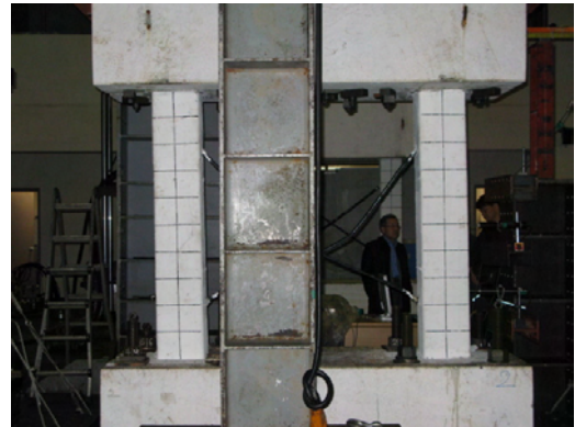
Fig. 9 Test result for the CR-2 specimen
