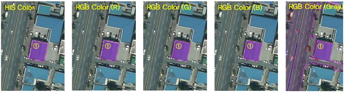
Figure 15. building area extracting result by color model(building① of study area(b))
