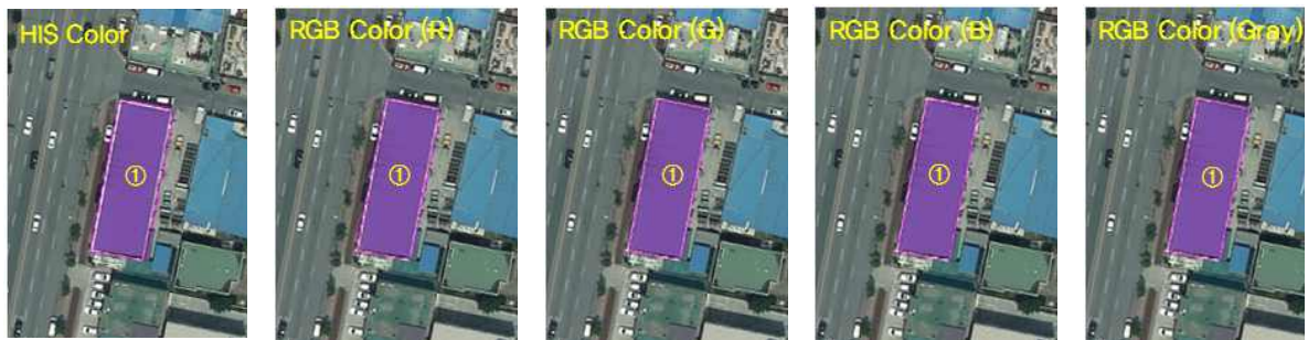
Figure 12. building area extracting result by color model(building① of study area(a))
