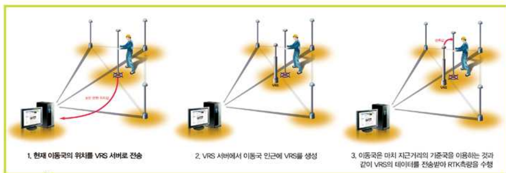
Figure 3. Principle of the VRS survey ( http://gps.ngii.go.kr/vrs/gps_vrs.asp )
