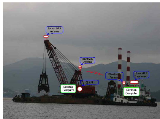
Figure 2. Arrangement of equipments in Grab dredger
