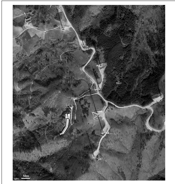
Fig. 4 Layout of wind turbines along access roads in the Yeongyang Wind Farm (source: Daum map)
