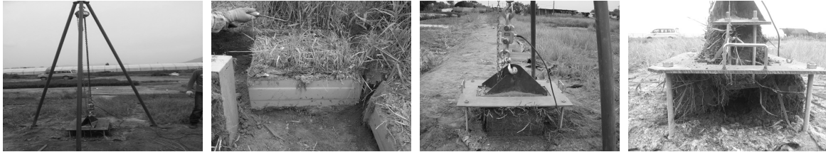
Photo 3. instrument of shear resistance stress test and cast (a) instrument of shear resistance stress test (b) vegetation in cast (c) before a shear resistance stress test (d) After shear resistance stress test
