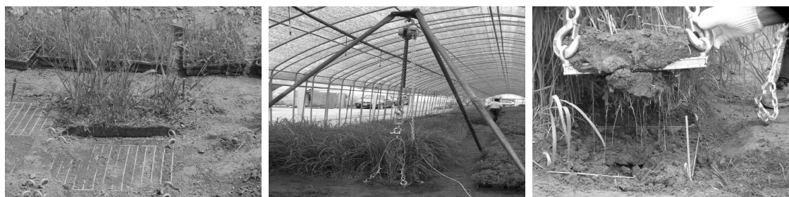
Photo 2. Instrument of Pull-out capacity Test and Test (a) Vegetation for test (b) Instrument of Pull-out capacity Test (c) After Pull-out capacity Test
