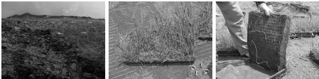
Photo 1. Mat-type Sod (a) Soil Erosion (b) Mat-type Sod (c) bottom of Mat-type Sod
