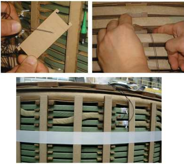
Fig. 2. Installation of the optical fiber sensor.
