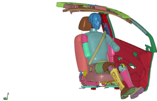
Fig. 2 Simulation model for side impact(EUROSID II)
