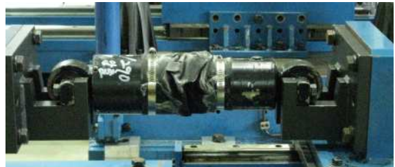
Fig. 11 Lateral damper of subway vehicle
