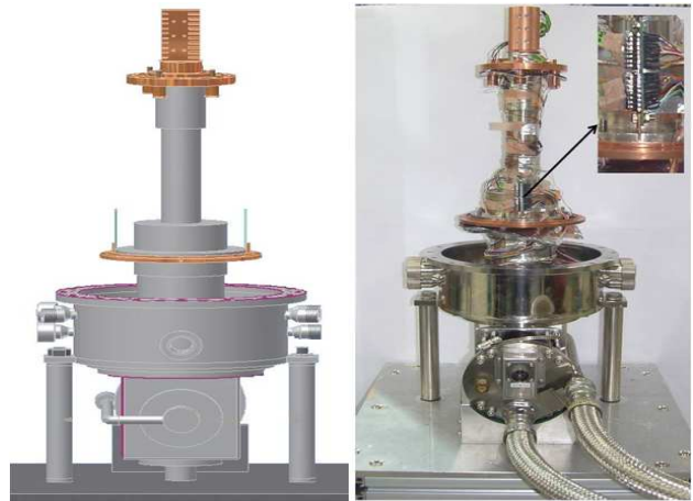
Fig. 7 3D-modeling and photo of calibration system
