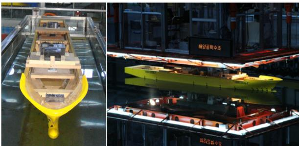
Fig. 6 Photographs of captive model test
