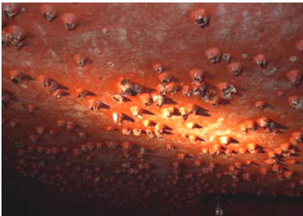
(b) Barnacle on the hull
