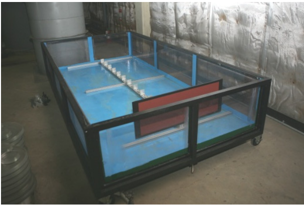
Fig. 5 Sea water deposition of painted plate
