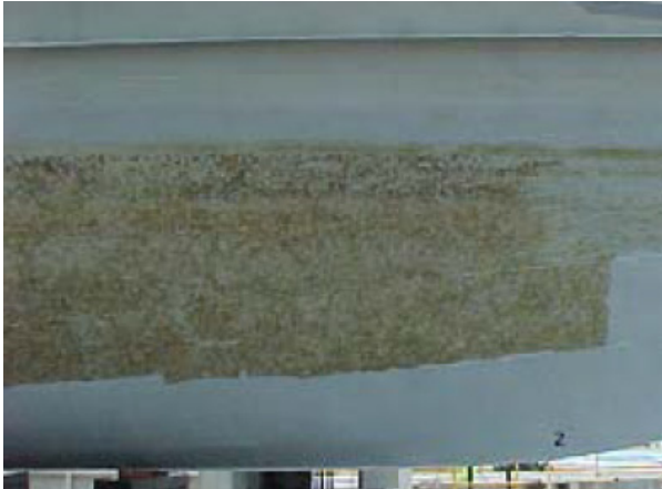
(a) Slime on the hull
