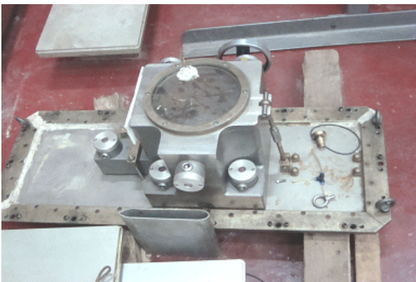
Fig. 6 Six-component force balance for drag measurements
