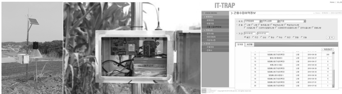
Fig. 2. Remote-sensing sex pheromone trap for capturing M. separata adults (left: complete set, center: control unit and power, right: webpage for the signal output).
