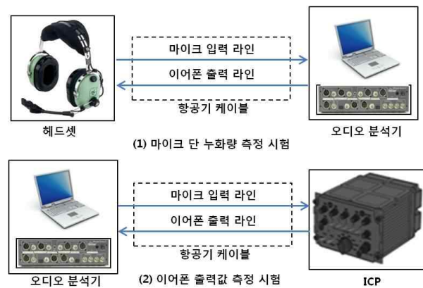
Fig. 10. Block diagram for measuring the amount of crosstalk in wire harness assembly
