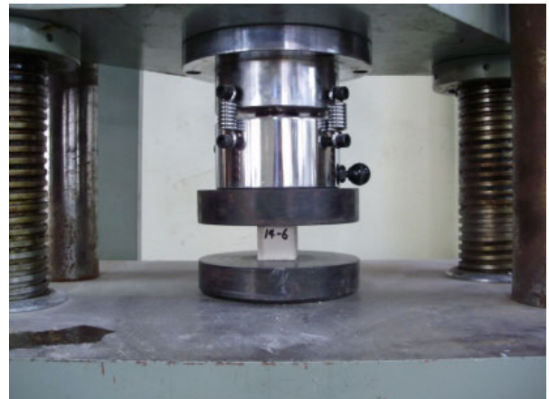
Fig. 5 Compressive Strength Test of Mortar Cube (KS L 5105)
