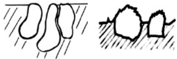
Low Noise Porous Pavement      Micro Surfacing Pavement
