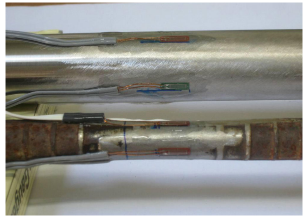
Fig. 4 Gauges Installation to Invar and Mild Steel
