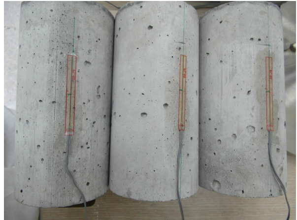
Fig. 6 Gauges Installation to Concrete Specimens (sample)
