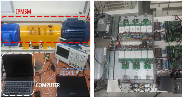
Fig. 7 Experiment set of proposed Full-Order Flux Observer and Power conversion set
