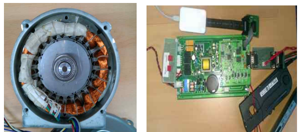
(a) PM synchronous motor (b) Control board
