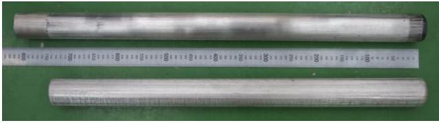
Fig.14 Butted tube after butting process
