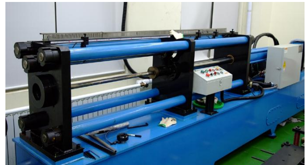
Fig.12 Test rig for tube butting process
